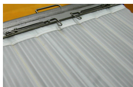
Diastar filter installed on filtrate drainage system
